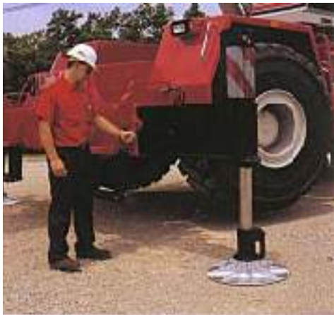
Fully Extended Outriggers 22' 0" (6.71 m) spread
