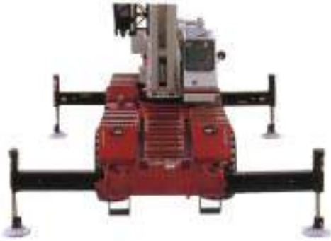
Fully Extended Outriggers 22' 0" (6.71 m) spread
